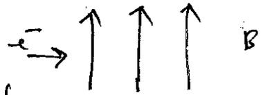
a) electron will experience a centripetal force which makes the electron move in a circular path into the page.
